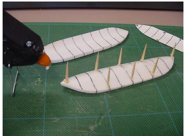
10. Turn this over and insert the spars into the underside of the upper elevator, doing the back row first and then the front, trying not to go all the way through the foam. Anchor with glue.
