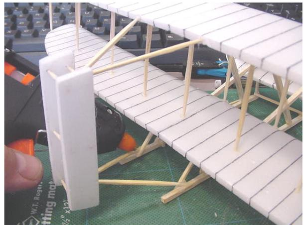
22. To make the propeller supports, use the template and mark and cut 5 toothpicks for each. Try to keep the assembly flat as it is glued.
